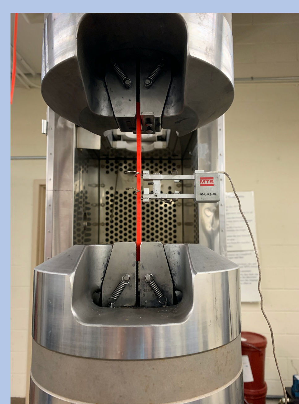
Figure 8: Tensile test being performed.
