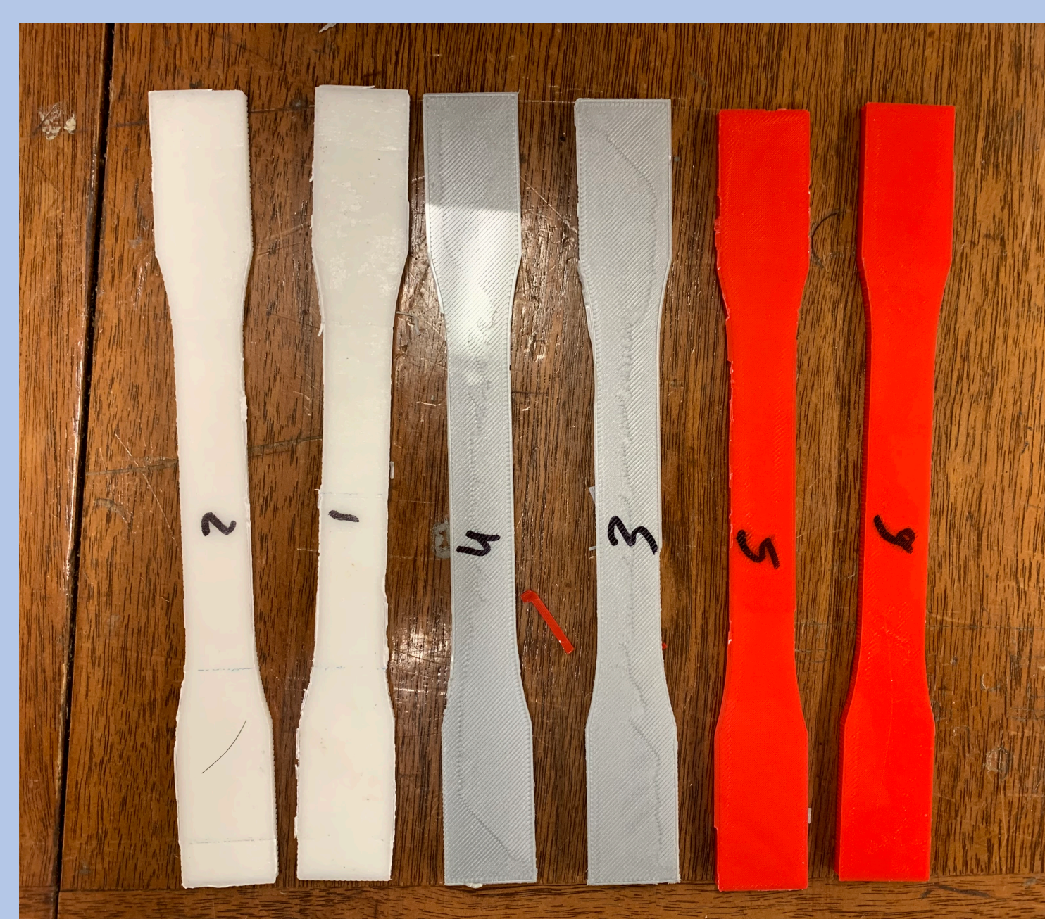
Figure 7: 3D printed specimen. 1 & 2 are ABS and 3,4,5 & 6 are PLA.
