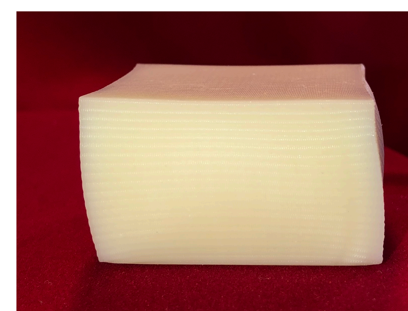
Figure 6 – 3D printed solid showing test-rig induced skewing
