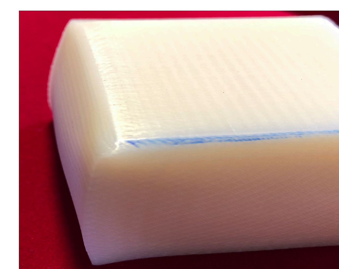
Figure 5 – Close up showing corner distortions on lab tested solid
