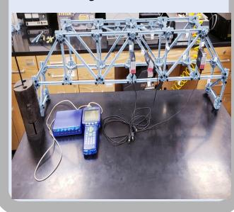
Methods & Findings The goal is to find the internal forces in the frames and observe the behavior of the bridge before collapse. For that purpose, different load and specific material were used. The theoretical part involved the use of method of joints, which is sum of all forces along X and Y equal to zero
