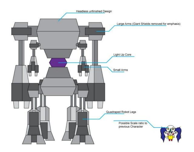
The Bulk of the Project would be constructed out of Cardboard with the center being plastic film. The "Core" a crystal ball prism flanked by LED lights powered by an enclosed Auduino.
