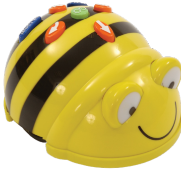
Figure 7: A general view of Bee-Bot with their commands on the top.
