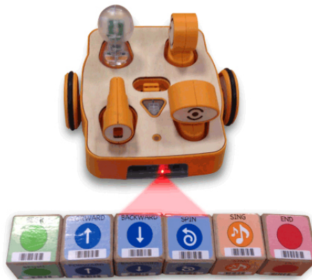
Figure 9: KIBO robot tool with the main blocks reading the code bar by infrared (Elkin, M., Sullivan, A., Bers, M. U., 2016).
