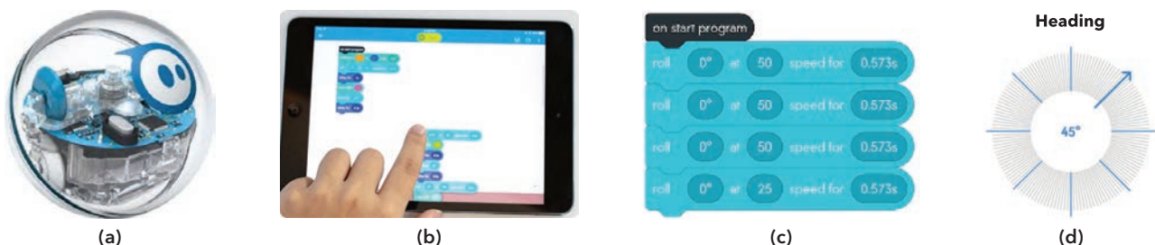
Figure 1. (a) The Sphero robot, (b) programming environment, (c) a sample program, and (d) interactive protractor for defining angles.
