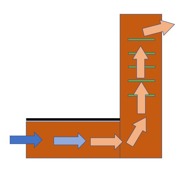
The solar dehydrators work using basic convection and the heat of the sun.
